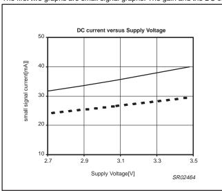
Figure 3. DC current vs. supply voltage
